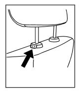
To raise a front seat head restraint, pull up on the restraint. To lower it, press the button, located on the top of the seatback, and push the head restraint down.
